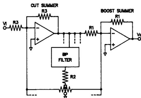
Fig. 8. Case 1—symmetrical constant-Q graphic equalizer topology.
