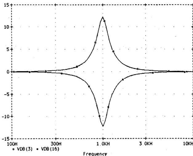
Fig. 9. Symmetrical boost/cut performance, case 1.
