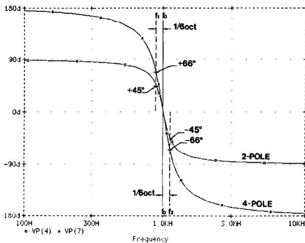
Fig. 20. Phase responses for two-pole and four-pole filters.
