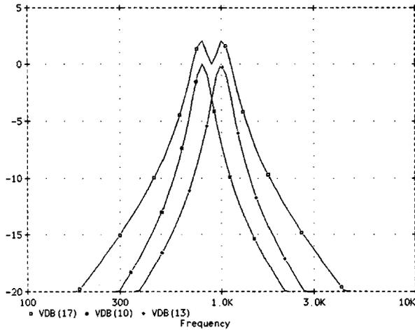
Fig. 18. Summed response of adjacent two-pole filters.
