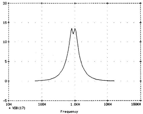
Fig. 22. Full boost results for adjacent two-pole filters.
