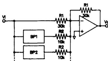
Fig. 14. Full boost “half-circuit” for +12 dB.
