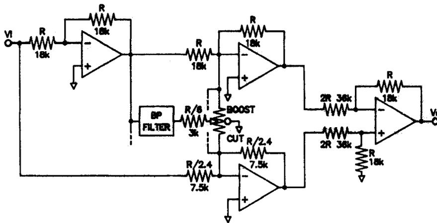
Fig. 10. Case 2—asymmetrical constant-Q graphic equalizer topology.
