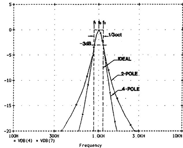
Fig. 15. Ideal two-pole and four-pole bandpass responses.
