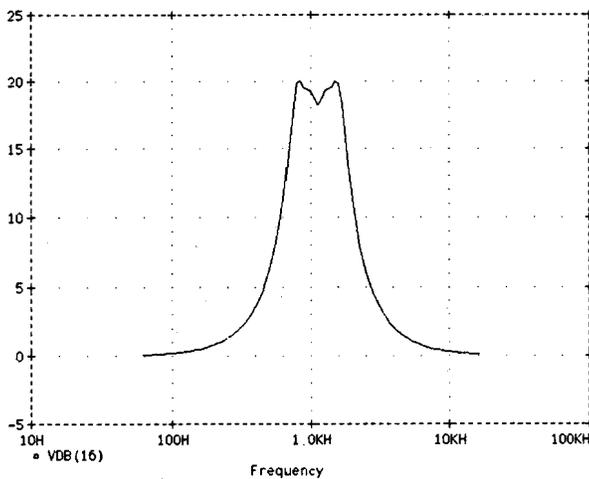
Fig. 37. As in Fig. 36, with sliders boosted 12 dB.
