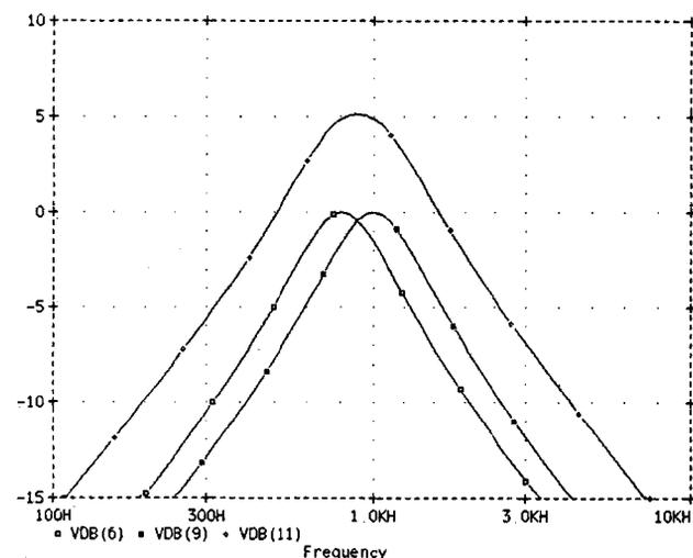
Fig. 27. Summed response of bandwidth degraded adjacent sections.
