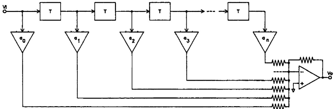
Fig. 13. Transversal filter graphic equalizer.
