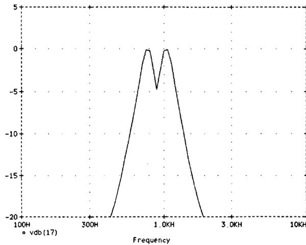
Fig. 19. Summed response of adjacent four-pole filters.
