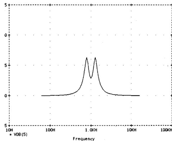
Fig. 38. Two alternate sliders boosted 6 dB.
