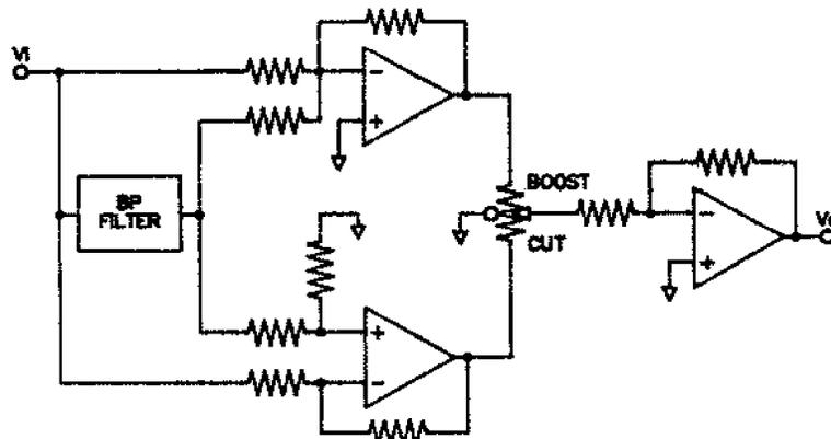
Fig. 12. Alternate asymmetrical constant-Q topology.
