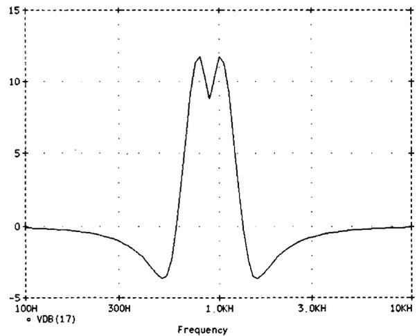
Fig. 23. Full boost results for adjacent four-pole filters.
