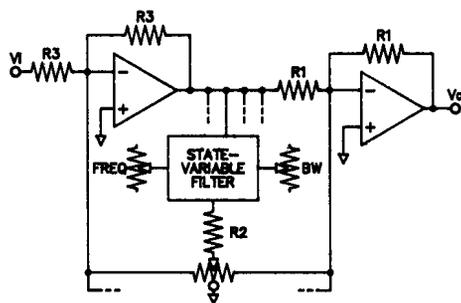
Fig. 7. Parametric equalizer topology.
