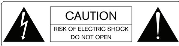
To reduce the risk of electrical shock, do not open the unit. No user serviceable parts inside. Refer servicing to qualified service personnel.
